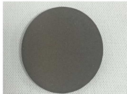
Micrometer-thick self-supporting hydrogen-containing boron target with \Phi=5.0 mm
