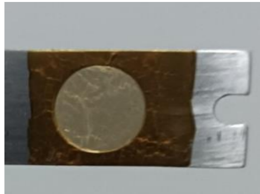
Nanometer-thick self-supporting 11 B target with \phi = 10.0 mm
